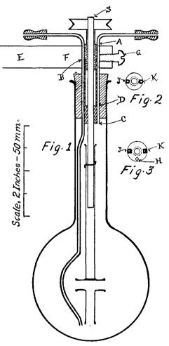
passes through a hole in the shaft and through holes in the stirrer. The shaft, S, is of 1/8 in. drill<sup>\*</sup> rod and carries a pulley of suitable size. The inlet and outlet tubes are bent as shown and carry enlargements so as to make convenient joints with rubber tubing.
